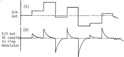
8. If the other signal input to the Ring Modulator carries an audio-frequency signal, that signal will be modulated by the voltage fluctuations of 7b above to produce a series of "events":
