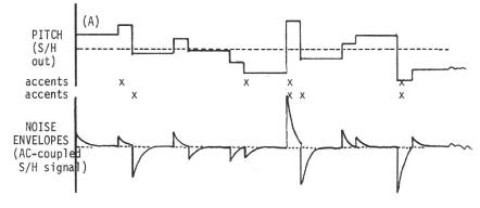
Note that the points of maximum amplitude in (b), the voltage which governs the Ring Modulator output volume, do not necessarily coincide with points of maximum amplitude in (a), which governs the pitch of the melodic sequence. The b\_ voltage corresponds much more nearly to the distance between successive voltage steps in waveform a. than it does to the absolute amplitude of any individual step. In mathematical terms, it is an approximation of the first derivative of waveform a.
