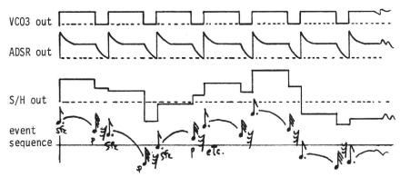
The diagram should make clear why this is happening. Changing the pulse-width now will change the rhythmic "feel" of the pitch-sequence. The second pitch in each envelope can be made to "disappear" by shortening the final decay (i.e. "release") time or by shortening the pulse-width to minimum. (There is at least one other way of doing this; figure it out and send us a note about it.)
